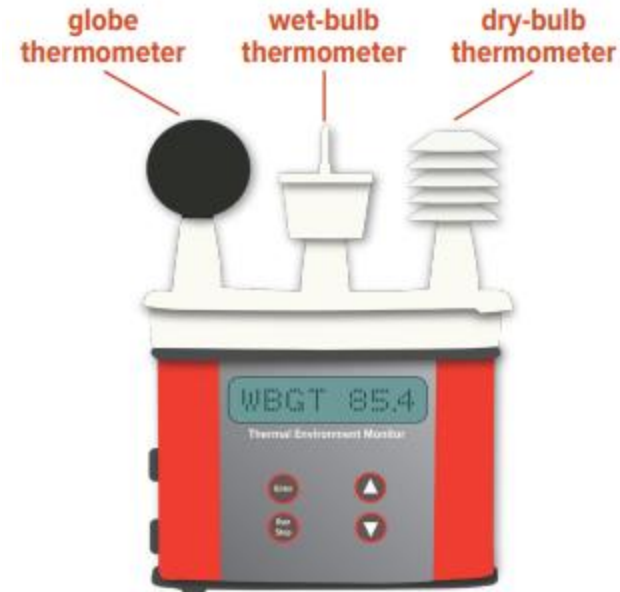
Example of WBGT Equipment
