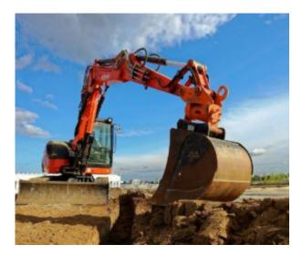
An excavation is any man-made cut, cavity, trench, or depression in an earth surface formed by earth removal. The trench is a narrow excavation (in relation to its length) made below the surface of the ground. In general, the depth is greater than the width.
