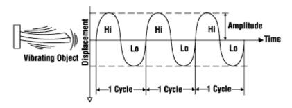
Figure 1 - Representation of the Measures of Vibration Exposure
