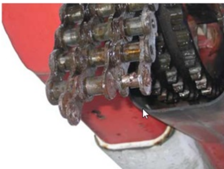
Photo 4: Broken section of boom actuating chain (photo courtesy of OSHA).
