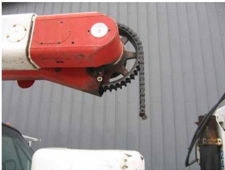
Photo 2: Broken boom actuating chain (photo courtesy of OSHA).
