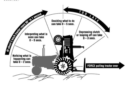
Factors that cause a tractor to tip over backward depend upon the load and the height of the hitch from the ground.
