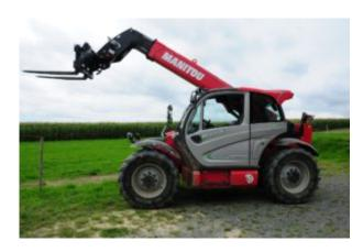
The Telehandler is a versatile piece of equipment found on most every job site. These unique machines can lift up to 10,000 loads and extend outwards 30 to 40 feet. Because of the size and power of this machine the safety and training of for this equipment is very important.
