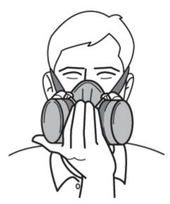
Figure 4: Positive pressure fit check
