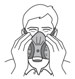
Figure 3: Negative pressure fit check
