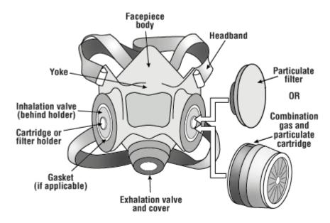
The basic parts of a typical half-facepiece respirator are shown.
