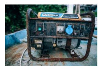
A 35-year-old man was found several hours after he died inside a barn he had been cleaning. He had been using a pressure washer with an 11-horsepower gasoline engine. He had apparently been working alone for about a half-hour before he collapsed. The doors and windows of the building were closed. The medical examiner determined he had died of carbon monoxide poisoning.
