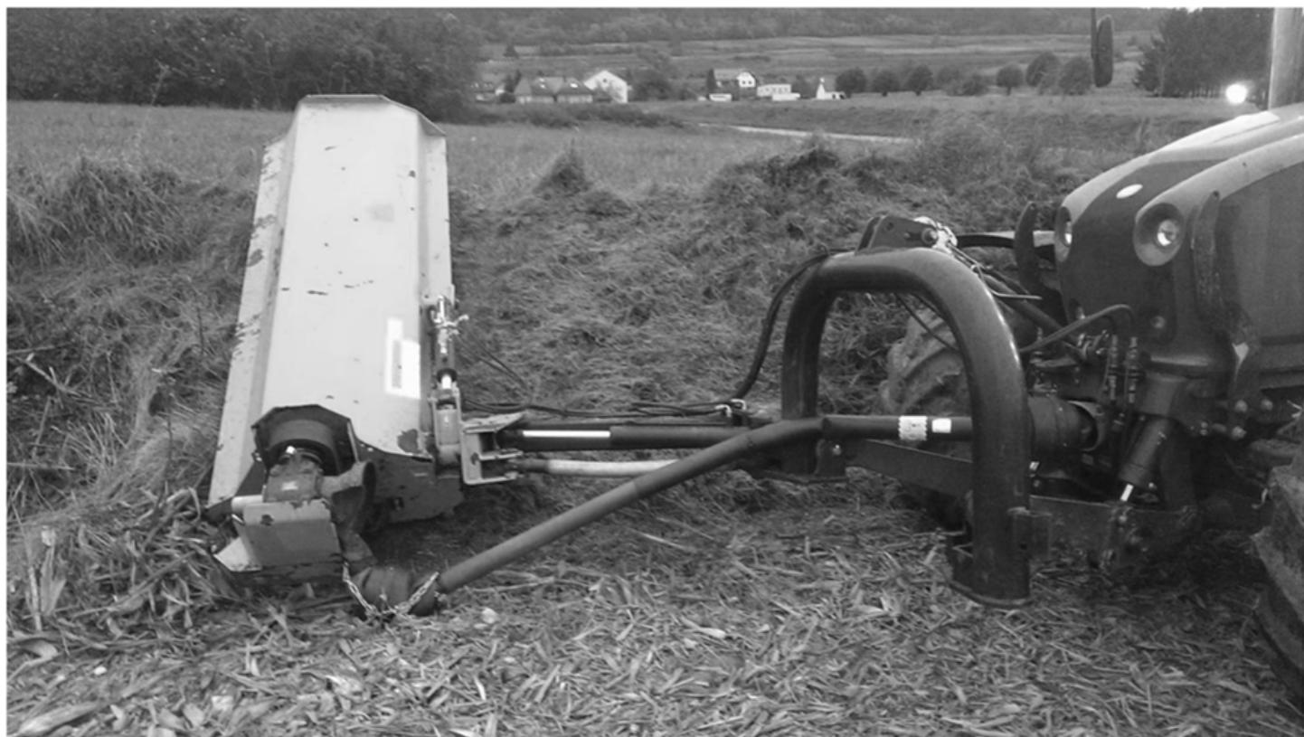
The Power Take-Off (PTO) shaft is operating without a full protective guard in place, leaving rotating components dangerously exposed. This creates a serious entanglement hazard for anyone working near the machine, especially when clothing, limbs, or loose objects can be pulled in quickly. The absence of guarding violates basic safety practices for operating agricultural equipment.
