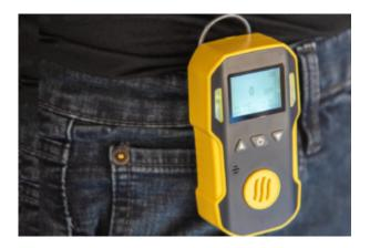
The use of portable gas detection devices helps ensure a workplace free from recognized hazards by providing employees working in potentially harmful environments the means to monitor their air quality. Harmful environments may include those with high levels of toxic or combustible gases or oxygen deficient or enriched air. Many of these conditions can't be detected by smell or sight and therefore require instrumental monitoring to view their levels.
