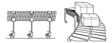
• Use a combination of lift tables and rollers to move materials horizontally and vertically.
