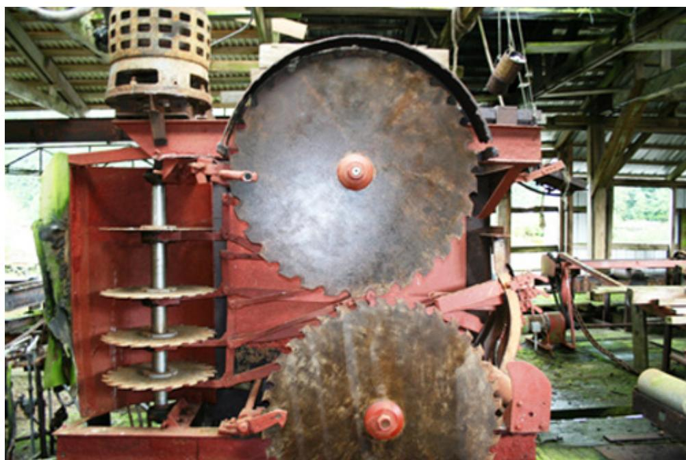
These brutes are seven-foot saws in a double circular mill arrangement. And they're not properly guarded.
