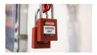
Lock Out, Tag Out (LOTO) is a safety procedure used in industry and research settings to ensure that dangerous machines are properly shut off.
