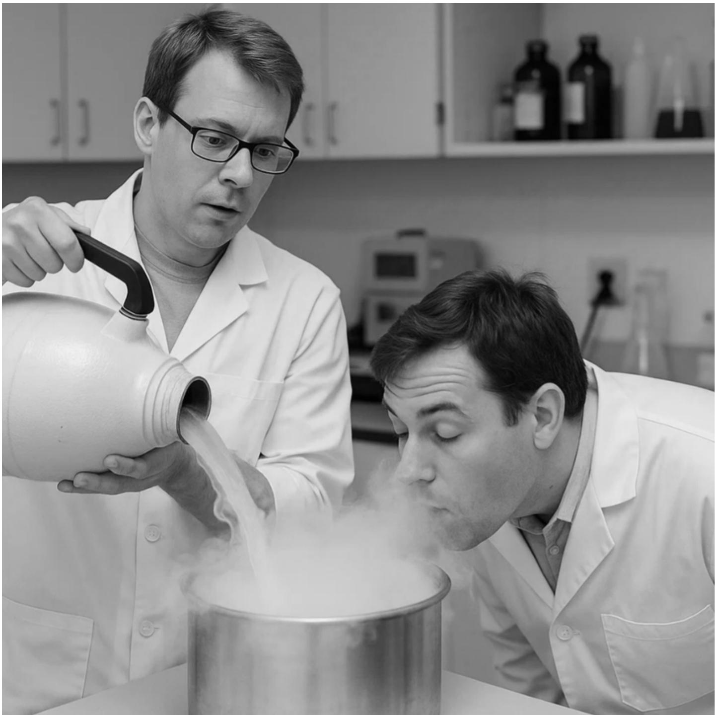
The man is placing his face directly over the vapor of liquid nitrogen while it's being poured. This is extremely dangerous. Liquid nitrogen vapor can displace oxygen, leading to dizziness or suffocation, and the extreme cold can cause cryogenic burns to the face or airways.
