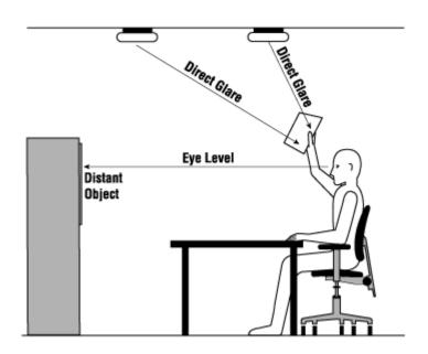
• To detect reflected glare, look at the task from your normal working position. Block the light falling on it from the front or above. If details are now easier to see, reflections are a problem.
