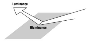
To determine reflectance, the light meter probe is placed on the test surface to measure light falling on the surface. Next, place the probe 5-7 cm away facing the surface to measure the light reflected from the surface. The following formula is used to calculate reflectance:
