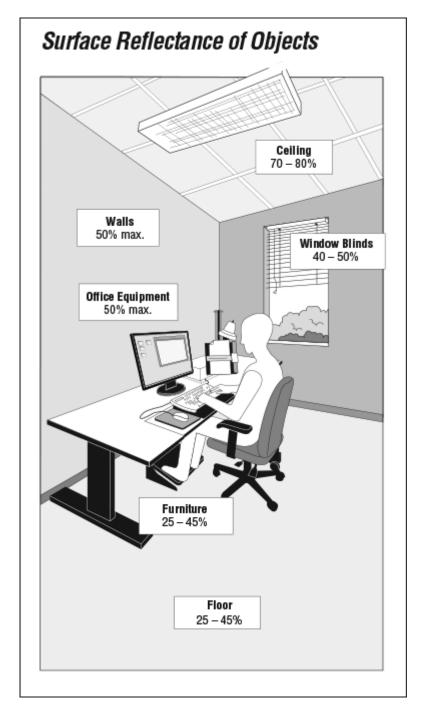
In addition, light fixtures that are too widely spaced or wrongly positioned can create shadows. Objects between the light fixture and work being done can block the light and cast shadows. Likewise, workers sitting with their backs to windows, with light fixtures directly overhead or to the rear, cast shadows on their own work surfaces.
