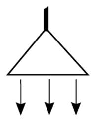
reflect light off the ceiling and other room surfaces. Little light is emitted horizontally meaning direct glare is often reduced. They are usually used in "clean" manufacturing areas.
