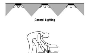
Localized-general lighting uses overhead fixtures in addition to ceiling fixtures to increase lighting levels for particular tasks.
