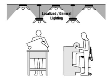
Local (or task) lighting increases light levels over the work and immediate
