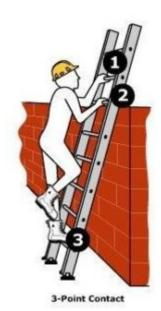
Always make sure the ladder is tied or secured correctly before using. When climbing up or down, always:
