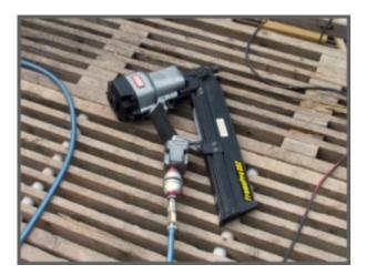
**4. Single Actuation Triggers** which like contact triggers, fire a single nail when the safety contact and trigger are activated in any order but also fire a second nail by
