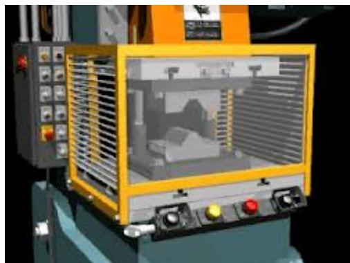
(Note: The machine guard in our "Spot the OSHA Violation" quiz above is also a fixed guard; but its openings are too wide to keep a worker from reaching into the guard and making contact with the point of operation.)
