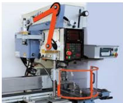
4. Self-adjusting guards in which the size of the opening in the barrier adjusts to accommodate the stock, e.g., enlarges to allow larger stock to enter
