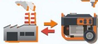
Transfer switches, whether manual or automatic, **allow** you to choose between **utility power** or **backup generator power**
