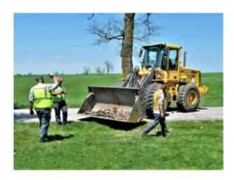
A machine operator was killed when he was run over by a front-end loader at a city's salt stockyard. The victim, employed by a liquid de-icer company, was walking around the loader working area. An equipment operator backed the loader out of a storage shed and struck the victim, who was not wearing a high-visibility safety vest. The loader was lacking two side-mounted mirrors and there was no radio communication between the victim and the city's equipment operators.
