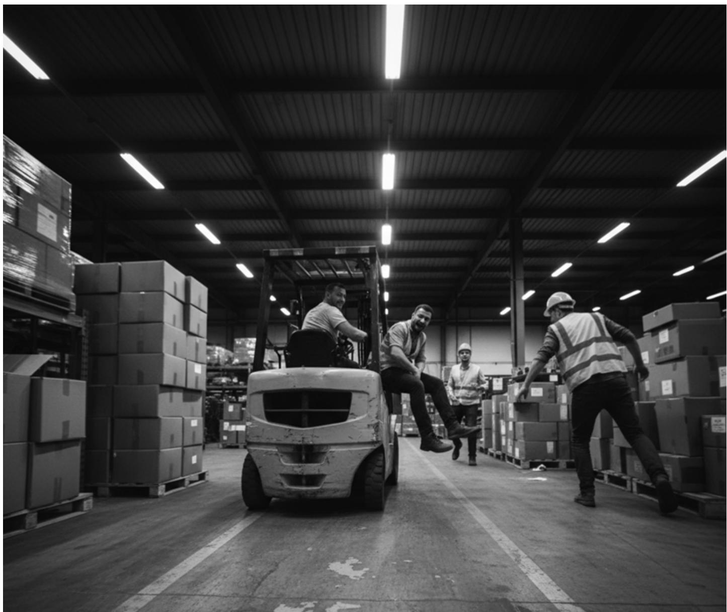
Workers are riding on a moving forklift, which is strictly prohibited. Forklifts are not designed for passengers, and this behavior puts both the riders and surrounding workers in immediate danger. Additionally, other workers are walking in close proximity, potentially within the forklift's rear swing radius—commonly known as the danger zone.
