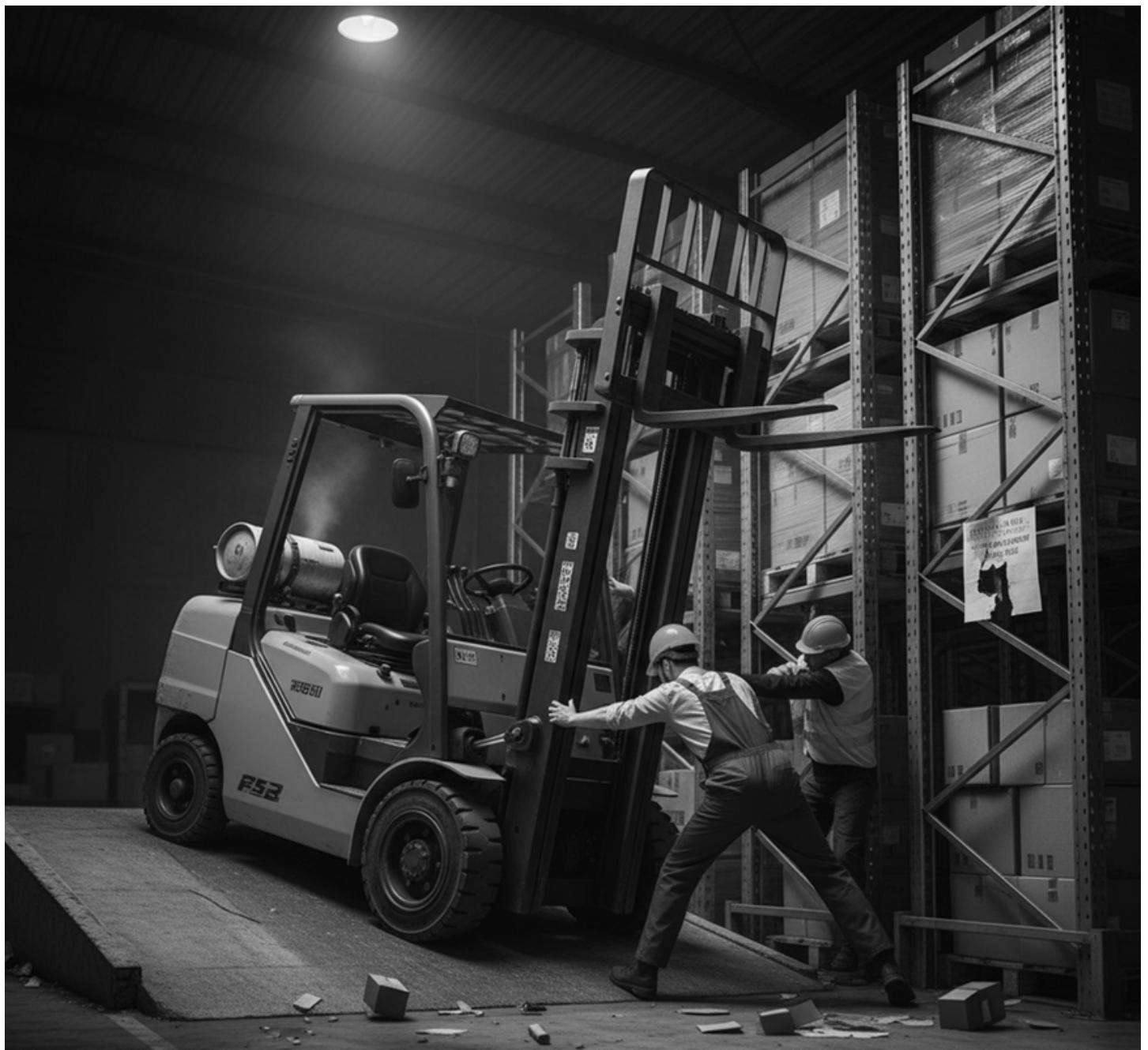
This image shows a forklift parked improperly on a ramp or incline, with the forks elevated and workers dangerously close to the equipment. One worker is physically touching the forks, and another is standing in the fall zone. Elevated forks create a
