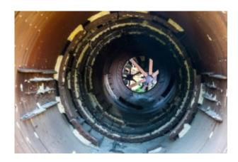
A fitter went into a concrete batching plant to do some repairs while the plant was still in use. As the sand he was standing on was discharged from the hopper into a mixing vehicle he was sucked down, buried by the sand and consequently asphyxiated.
