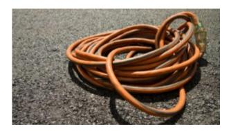
Even a simple extension cord needs to be looked after. It's a shock or fire hazard when deteriorated, worn-out or used improperly.
