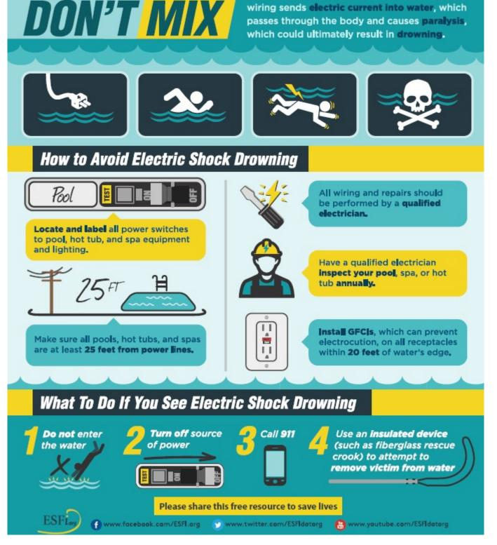
Electric Shock Drowning (ESD) severely injures and kills people every year. ESD occurs when faulty wiring sends electric current into water, which passes through the body and causes paralysis, which could ultimately result in drowning.
